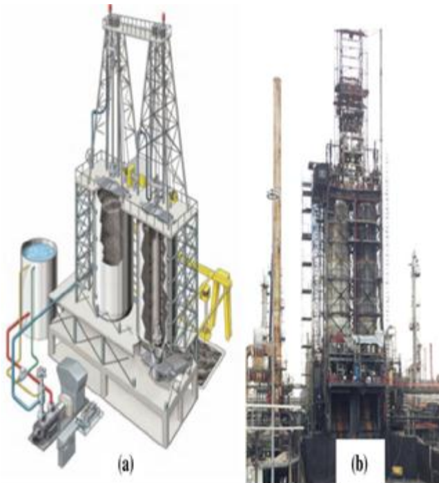
Fig1-Delayed coker operation, schematic (a) and delayed coker (b)
